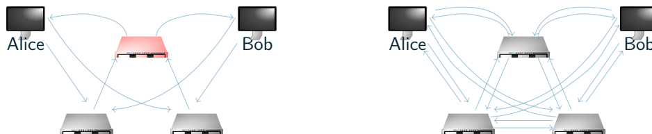
Figure 3: A Mixnet with a bottleneck (in red, left), and a Mixnet with free routes (right.)
